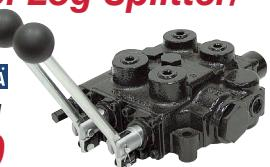
• Brand new PRINCE Model RD522CC-EA5A4B1 control valve. Ideal for use in log splitters equipped with a log lift. First spool has a pressure release detent on the spool-out position and springs to center on the spool-in position. Second spool is 3-position spring to center. Detent pressure preset to 1200 PSI, adjustment range 1000-2000 PSI.
